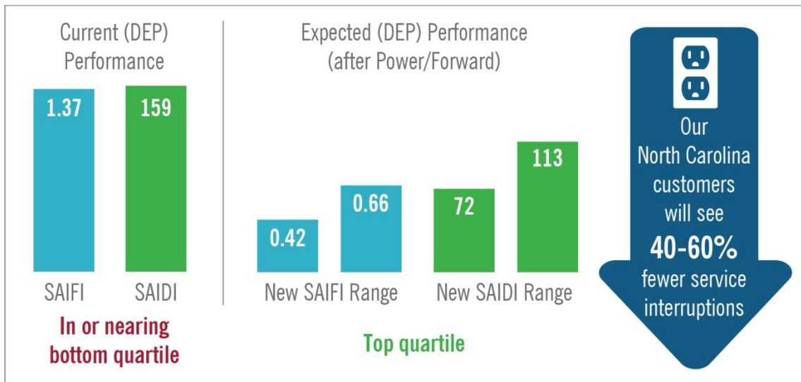
Figure 2 – This data reflects significant improvements that occur in Duke Energy Progress’ SAIFI and SAIDI reliability performance measures in NC after Power/Forward is implemented. (Ranges of improved performance are based on historic load and weather information and do not reflect any impacts from changes in weather severity or customer
